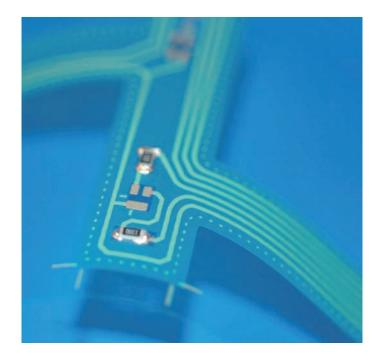
Conductive adhesives are usually thermally curing epoxy resin-based or UV-curing acrylate-based adhesives augmented with metallic or anorganic fillers.
