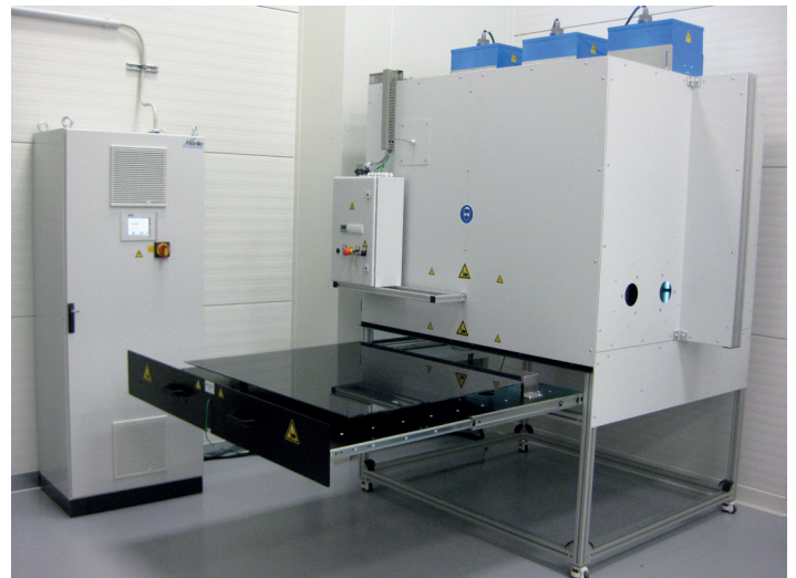
Irradiation chamber 1,1 m x 1,3 m
